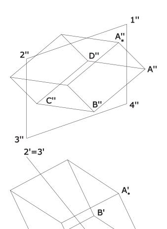
Construct the intersection of the prism and the plane of parallelogram. Show the visibility.
