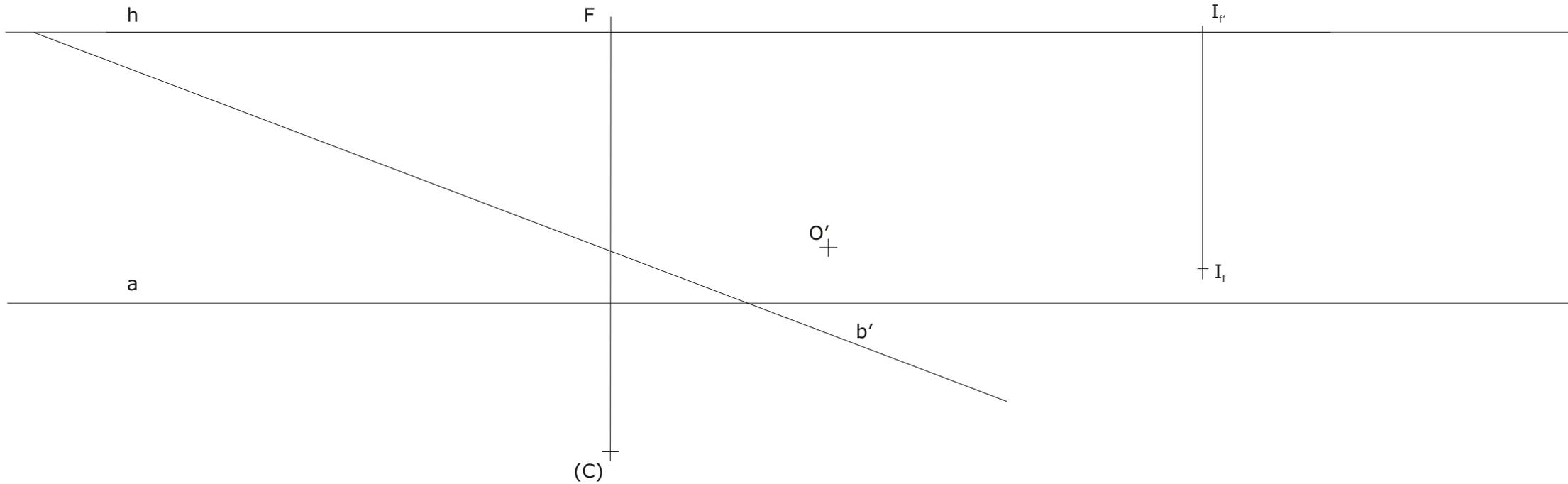
Represent a prism with regular hexagon base in perspective with vertical picture plane. The center of the hexagon is the point  $O$ , one of the sides lies on line  $b$ , and the height of the prism is 82 mm. Remove the lateral face, closest to the observer (centre of perspective). Show the visibility of the surface that consists of the base hexagon, lateral faces and the top face. Construct all shadows and shades at parallel lighting given by  $I_r$  and  $I_{r'}$ .
